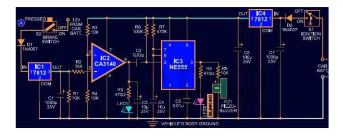
Brake failure indicator circuit that constantly monitors the condition of the brake and gives an audio-visual indication. When the brake is applied, the green LED blinks and the piezobuzzer beeps for around one second if the brake system is intact. If the brake fails, the red LED glows and the buzzer stops beeping[6].
